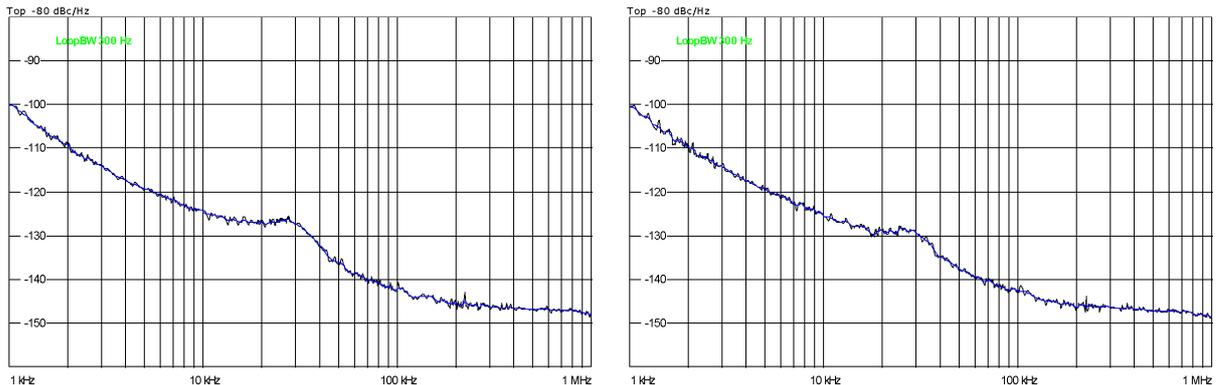
Fig. 1: Phase noise in units of [dBc/Hz] as function of the frequency offset for the setup of transceiver K3, transverter TR144H+40, and power amplifier BEKO HLV-600. The system power output has been about 400 W (left) and 550 W (right).
