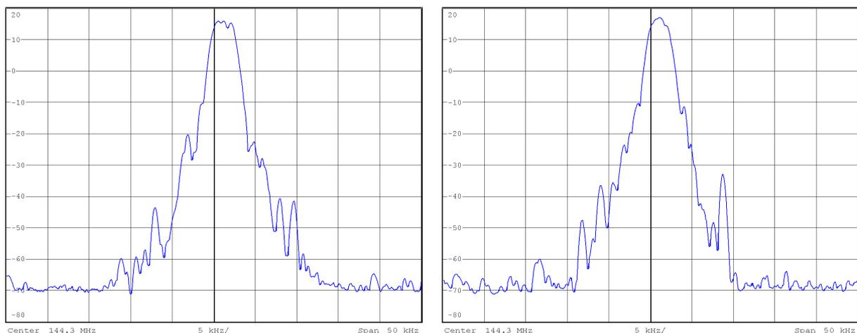
Fig. 3: Spectra of the transmitted signal amplitude in units of [dB] at 3 kHz bandwidth as function of the frequency offset when using mode SSB for the setup of transceiver K3, transverter TR144H+40, and power amplifier BEKO HLV-600. The system power output has been about 400 W (left) and 550 W (right).
