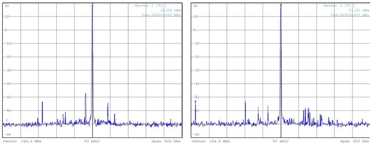
Fig. 2: Spectra of the transmitted signal amplitude in units of [dB] at 3 kHz bandwidth as function of the frequency offset when using mode CW for the setup of transceiver K3, transverter TR144H+40, and power amplifier BEKO HLV-600. The system power output has been about 400 W (left) and 550 W (right).
